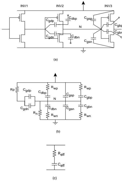
Figure 3 Capacitance model for device capacitance in power grid analysis
