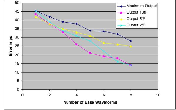
Figure 7. Obtained trade-off between delay model error and number of base waveforms for three loading and across all
