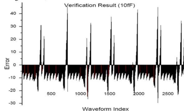
Figure 9. Delay model error when tested with 3500 test waveforms.
