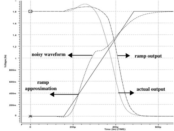
Figure 1. Signal waveforms due to capacitive shielding and coupling noise and their impact on gate delay model accuracy.
