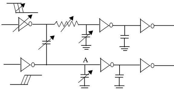
Figure 3. Interconnect structure to generate candidate waveforms
