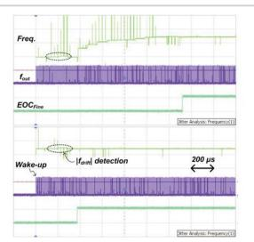
Figure 10.9.4: Measured locking transients after wake-up with (upper) a large frequency drift and (lower) a small frequency drift.
