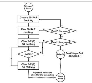
Figure 10.9.3: Lock procedure.
