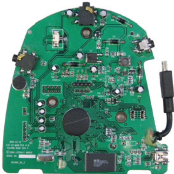
Fig 3. Talking Book’s PCB and 152 off-the-shelf components
