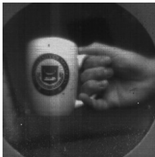
Figure 11. Sample image taken with the image sensor and GRIN lens, transmitted via Mbus.
