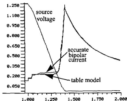
Figure 7. Waveforms of bipolar effect current simulated using accurate and table models
