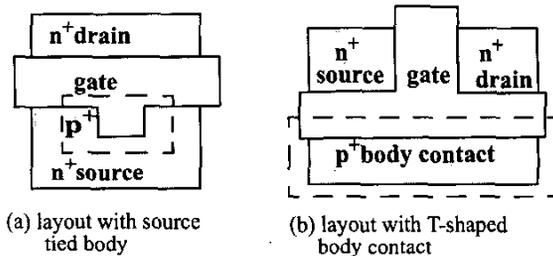
Figure 2. Layout of SOI transistors
