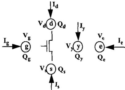
(b) electrical model of SOI transistor:
