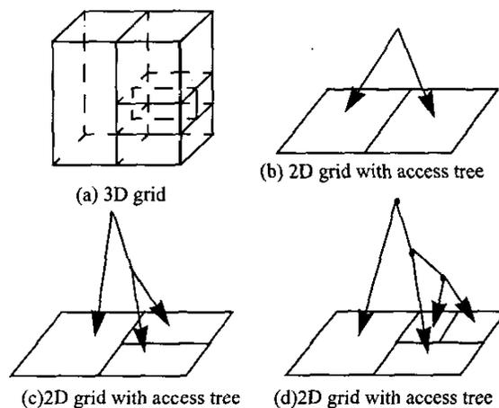
Figure 4. Construction of grid and binary access tree
