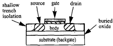
(a) structure of SOI transistor
