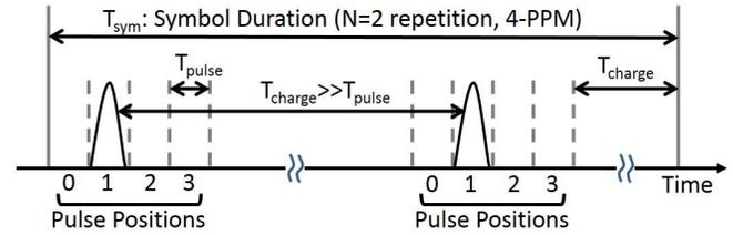
Fig. 5. N-repetition M-PPM modulation illustration.  $N = 2$ , 4-PPM example.
