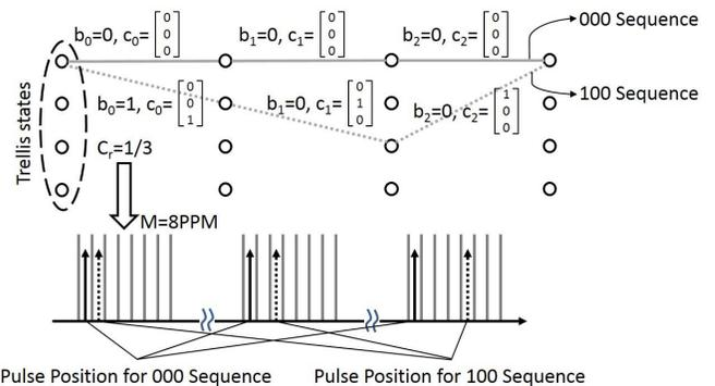
Fig. 8.  $\nu = 3$ ,  $C_r = 1/3$  coding example. M-PPM size is tightly coupled with  $C_r$ .  $M = 2^{1/C_r} = 8$  PPM is used.
