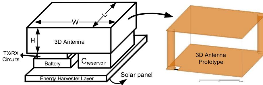
Fig. 2. Millimeter-scale stacked system (left) and 3D magnetic antenna (right) diagram.
