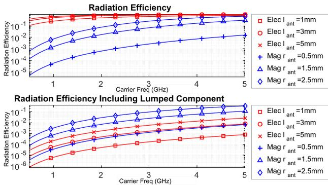
Fig. 3. Radiation Efficiency of Electric and Magnetic Dipoles.
