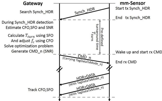
Fig. 6. Gateway guided synchronization and link adaptation.
