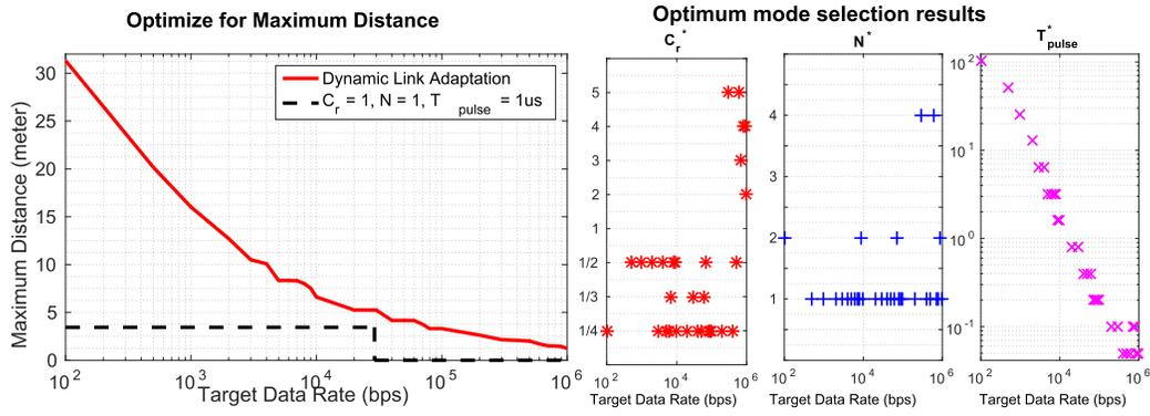
Fig. 12. Maximum distance objective link adaptation result.
