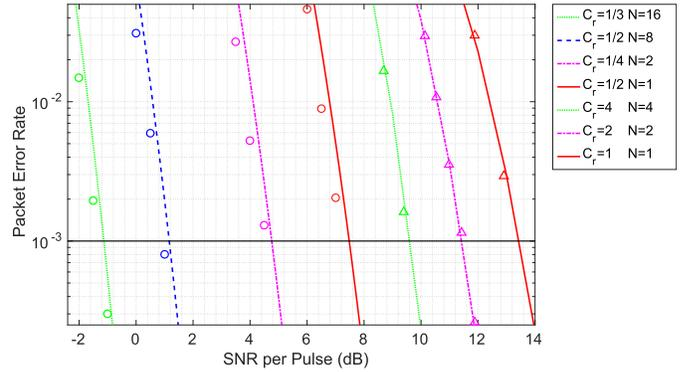
Fig. 11. Performance of modulation-coding scheme. Analysis for uncoded cases. Tight union bound for coded cases.
