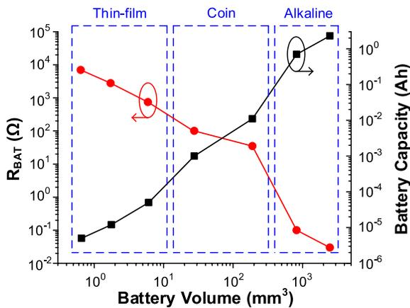
Fig. 4.  $R_{BAT}$  and battery capacity across battery volumes.
