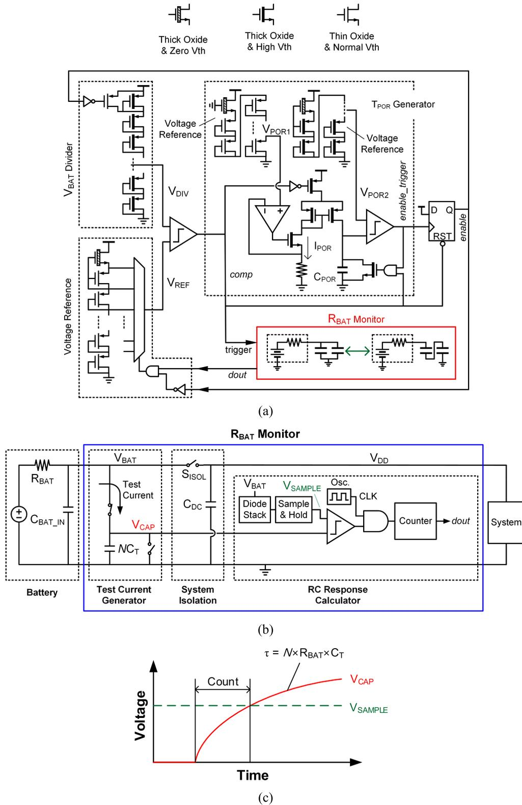
Fig. 11. Circuit diagram of AHBVS. (a) BVS. (b)  $R_{BAT}$  monitor. (c) Conceptual operation of  $R_{BAT}$  monitor.
