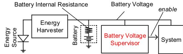
Fig. 1. IoT system with BVS.
