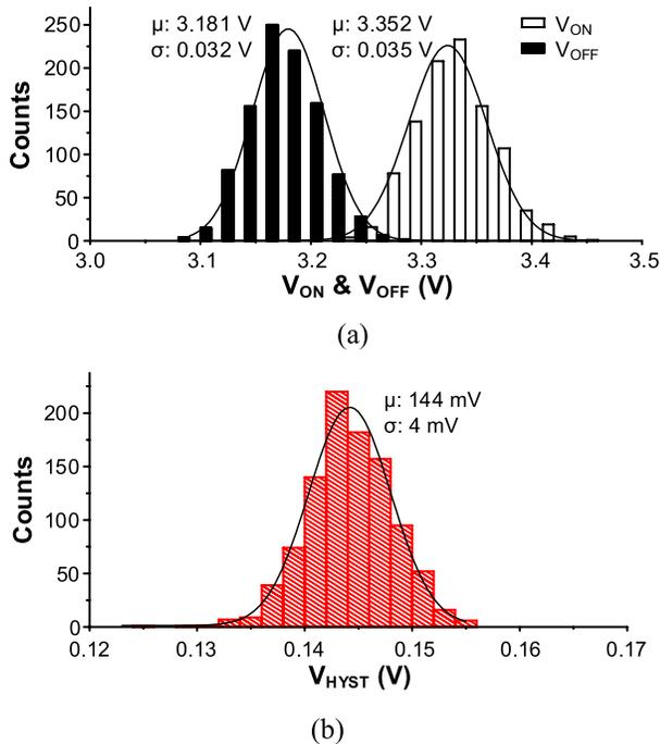
Fig. 7. Simulated impact of process variation and device mismatch on reset threshold voltages. (a)  $V_{ON}$  and  $V_{OFF}$ . (b)  $V_{HYST}$  ( $=V_{ON} - V_{OFF}$ ).
