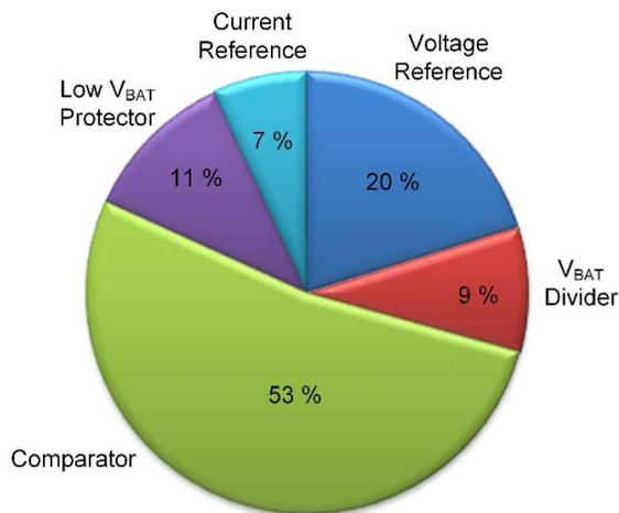
Fig. 25. Power breakdown of AHBVS.
