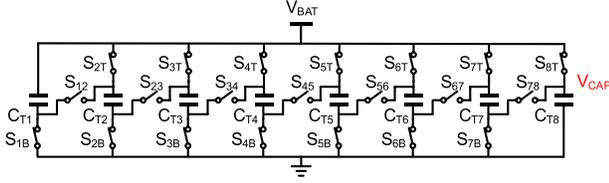
Fig. 12. Circuit diagram of test current generator.
