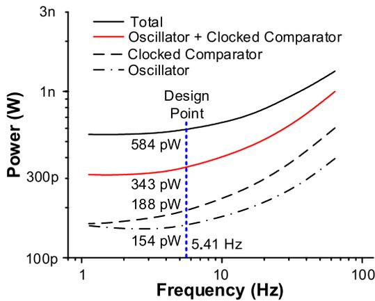
Fig. 28. Simulated LCHBVS power consumption breakdown across operating frequencies.
