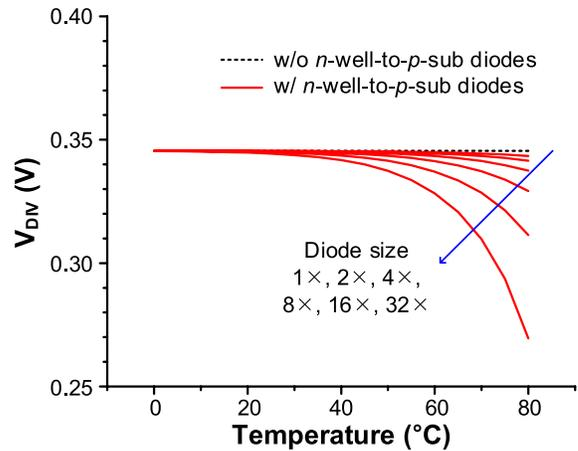
Fig. 21. Simulated effect of leakage current through n-well to  $p$ -subdiodes on  $V_{DIV}$  across temperatures.
