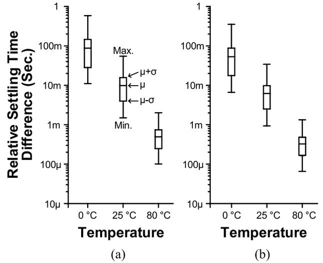
Fig. 10. Simulated relative settling time difference (settling time of  $V_{DIV}$ –settling time of  $V_{REF}$ ). (a) 3.8 V. (b) 4.2 V.
