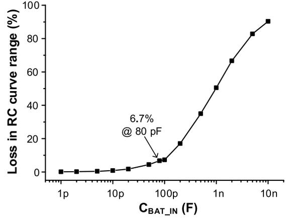
Fig. 17. Simulated loss in the RC curve range across  $C_{BAT\_IN}$ .
