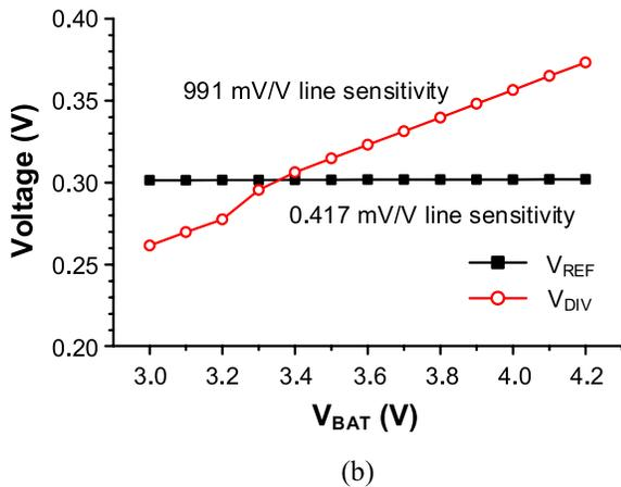
Fig. 20. Measured  $V_{REF}$  and  $V_{DIV}$ . (a) Temperature dependency. (b)  $V_{BAT}$  dependency.
