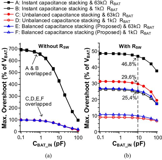
Fig. 14. Simulated overshoot on  $V_{BAT}$  (a) without  $R_{SW}$  and (b) with  $R_{SW}$ .
