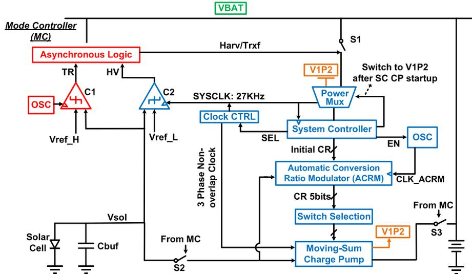
Fig. 10. Detailed architecture of discontinuous harvester.
