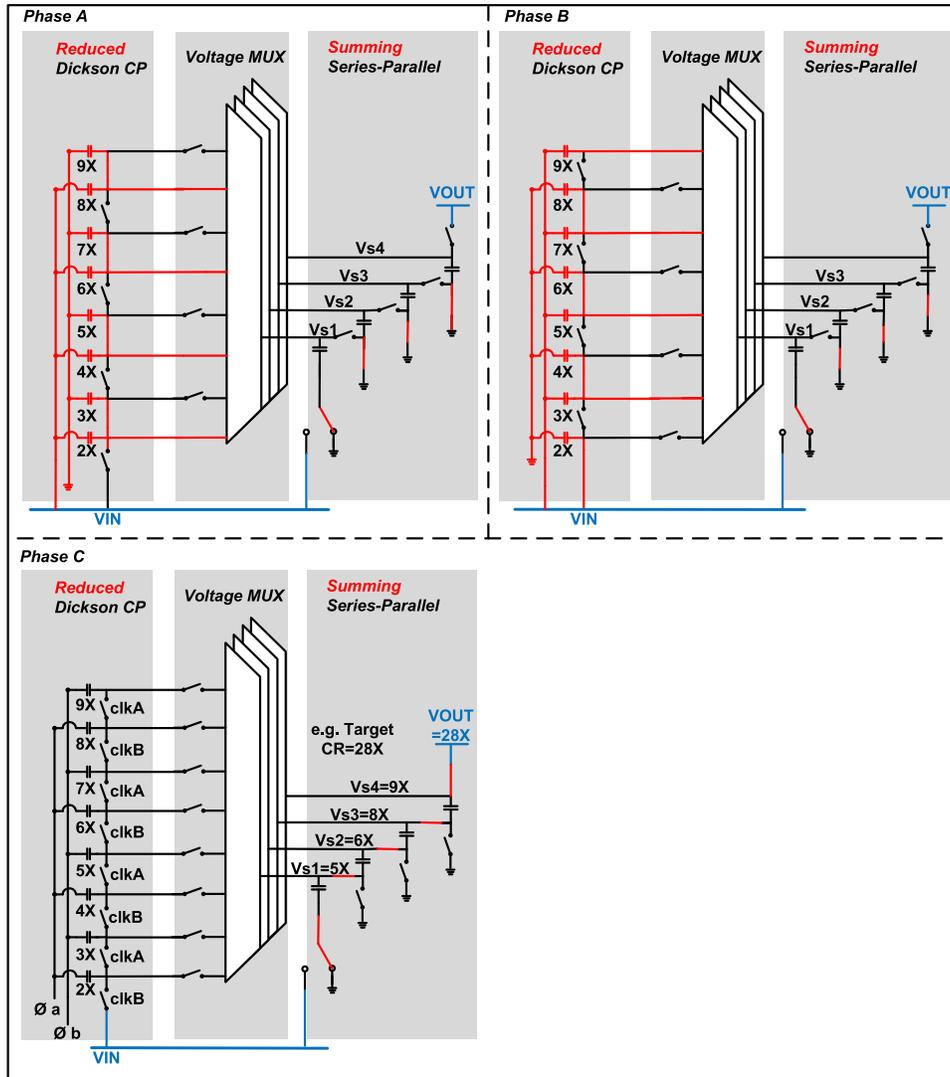
Fig. 15. Three-phase operation of moving-sum charge pump.
