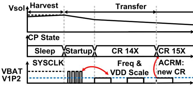
Fig. 11. Timing diagram of the discontinuous harvester.
