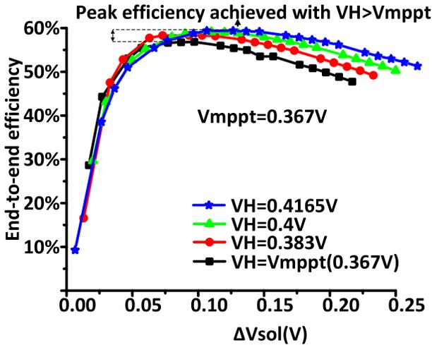
Fig. 7. Dependence of simulated end-to-end efficiency on  $V_H$ .
