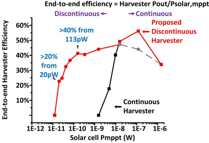
Fig. 25. Harvester measurements.
