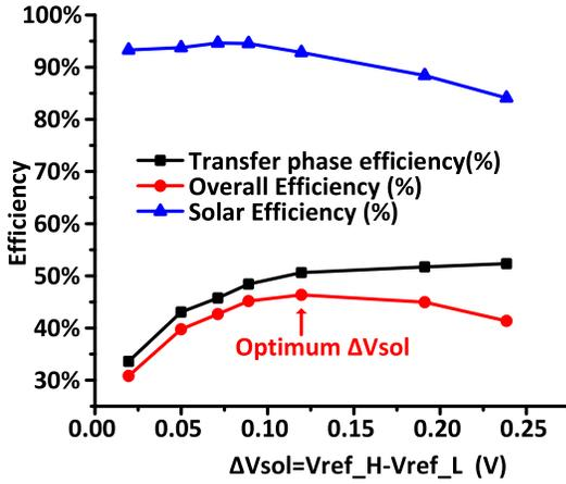
Fig. 26. Measured tradeoff between transfer phase efficiency and solar efficiency.
