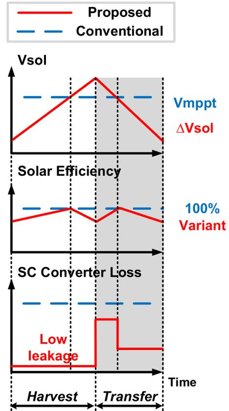
Fig. 5. Conceptual operation of discontinuous harvester.
