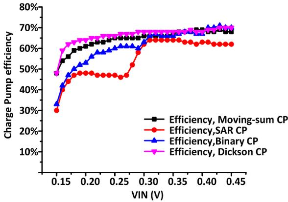
Fig. 19. Charge pump efficiency comparison based on simulation.
