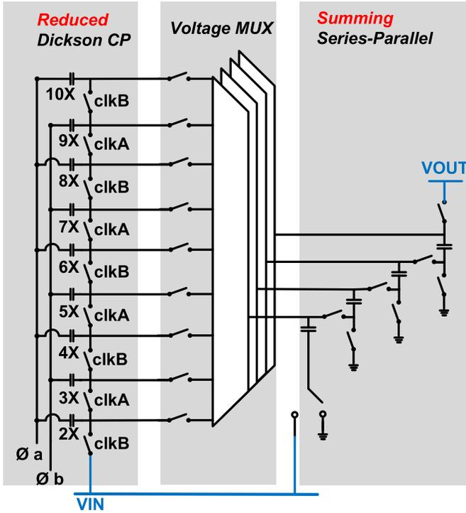
Fig. 14. Structure of moving-sum charge pump.
