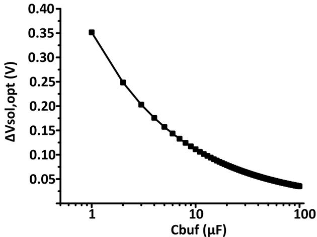
Fig. 8. Dependence of  $\Delta V_{sol, opt}$  on  $C_{buf}$  based on calculation.
