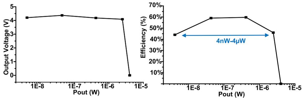
Fig. 24. Moving-sum charge pump measurements.
