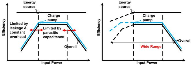
Fig. 3. Conceptual efficiency illustration of (a) traditional harvester efficiency and (b) proposed harvester.
