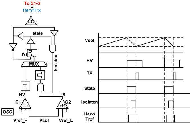
Fig. 21. (a) Circuit diagram of the mode controller. (b) Timing diagram.
