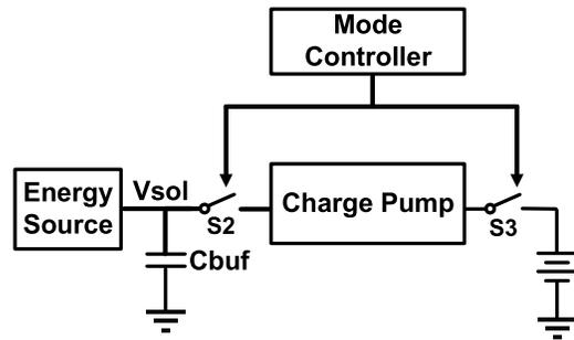
Fig. 4. Concept of discontinuous harvester.
