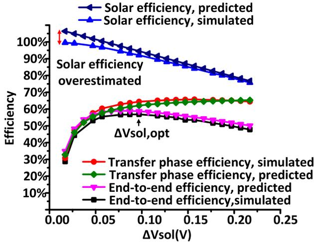
Fig. 6. Dependence of efficiencies on  $\Delta V_{sol}$  based on model prediction and simulation.
