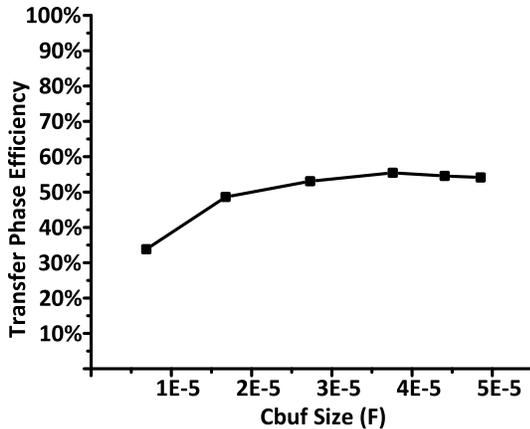
Fig. 27. Measured dependence of transfer phase efficiency on Cbuf size.
