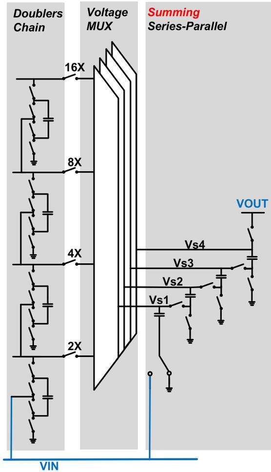
Fig. 17. Structure of binary charge pump.
