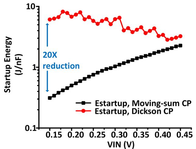
Fig. 16. Simulated startup energy comparison between moving-sum charge pump and Dickson charge pump.
