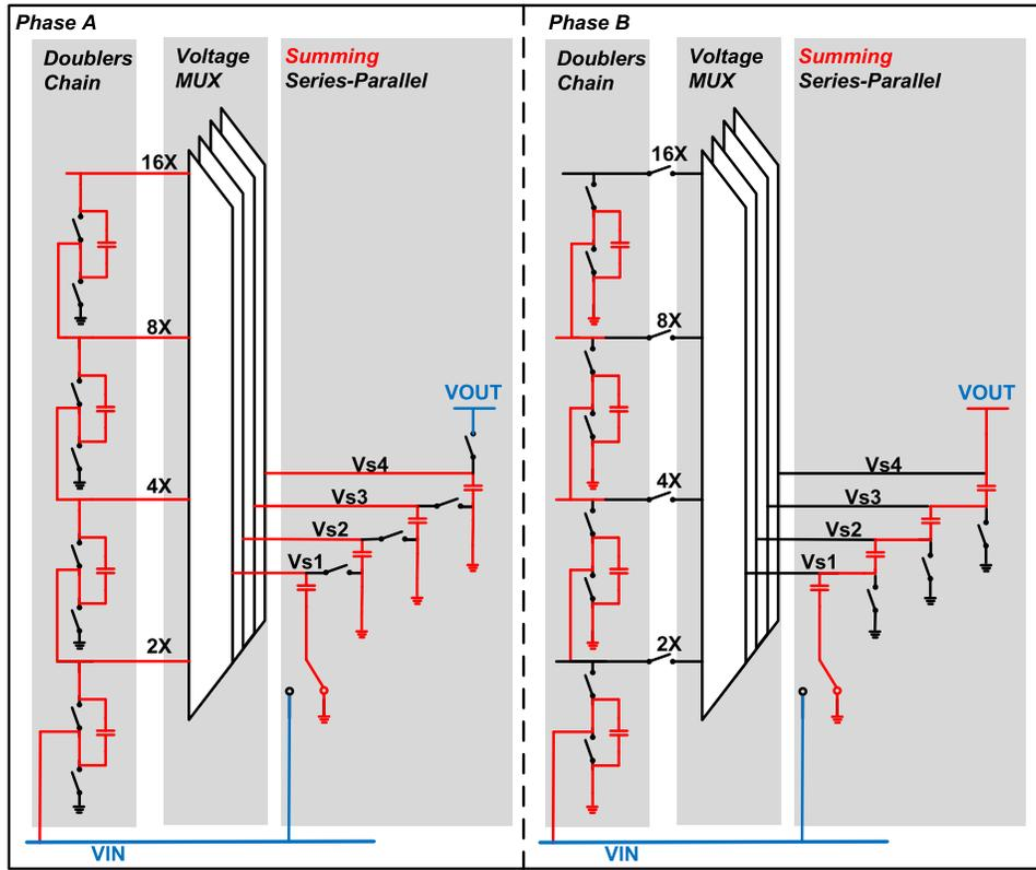
Fig. 18. Two-phase operation of binary charge pump.
