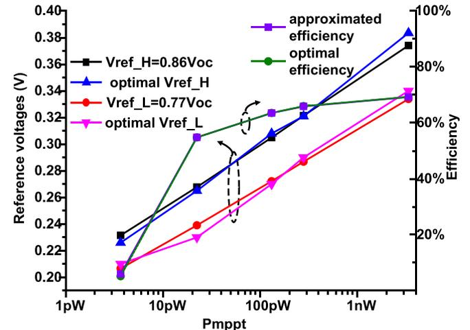
Fig. 13. Simulated end-to-end efficiency with approximated  $V_{ref\_H}$  and  $V_{ref\_L}$ .
