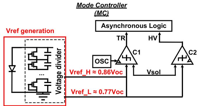
Fig. 12. Proposed reference voltages generation.
