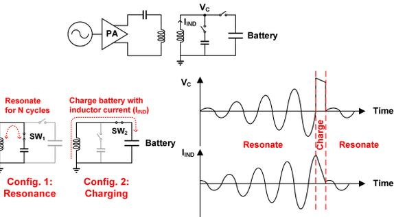
Proposed "Wireless power receiver and current-mode charger with optimal resonant cycle tracking" system
