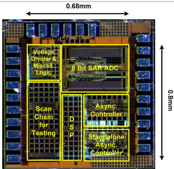
Figure 21.5.7: Micrograph of 0.18μm test chip (0.68mm × 0.8mm).
