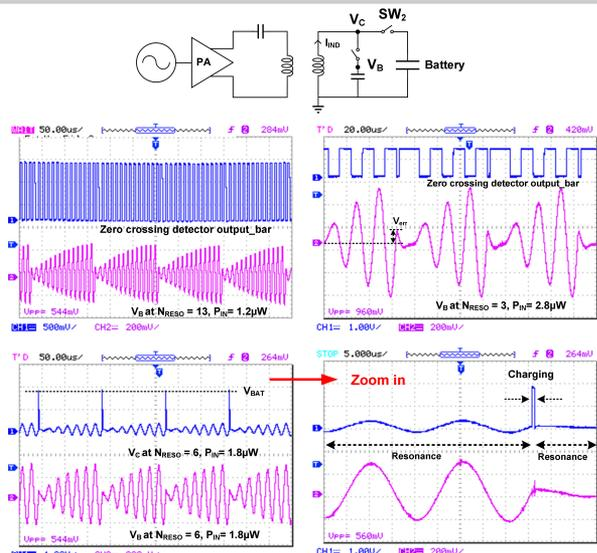
**Figure 21.5.5: Waveforms measured by oscilloscope.**
