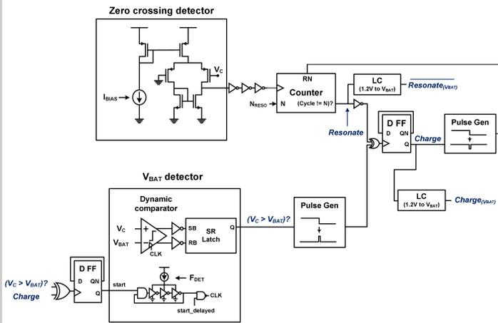
**Figure 21.5.3: A detailed circuit diagram of the wireless power receiver controller.**
