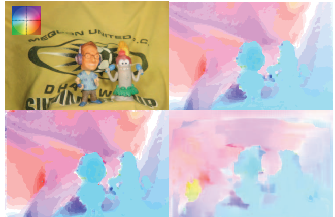
Fig. 2. Colored flow maps of ‘Mequon’ using different algorithms. Top-left: input previous frame and color legend; top-right: NG-fSGM, N = 3 ; bottom-left: fSGM; bottom-right: Lucas-Kanade.
