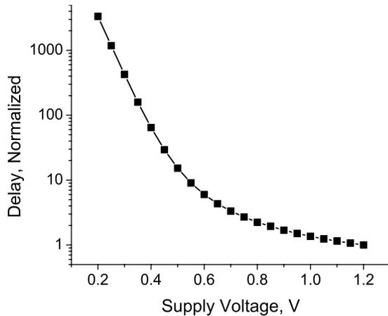
Figure 1. Impact of supply voltage scaling on delay.
