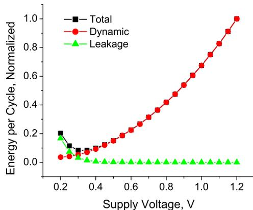
Figure 2. Impact of supply voltage scaling on energy.
