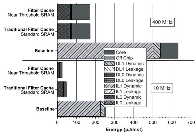
Figure 8. Filter cache energy breakdown for BitCount benchmark.
