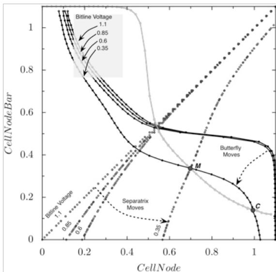
Figure 11. Evolution of 6T cell stability during write
