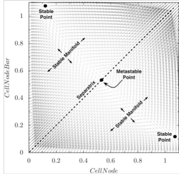
Figure 2. 45nm SRAM cell dynamical phase portrait
