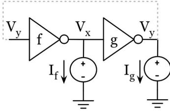
Figure 5. SRAM cell nullcline / butterfly equivalence
