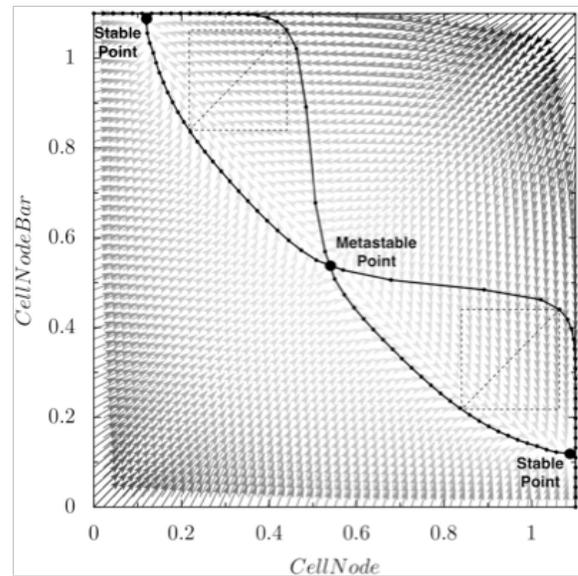
Figure 4. Nullcline trace of a 45nm 6T cell
