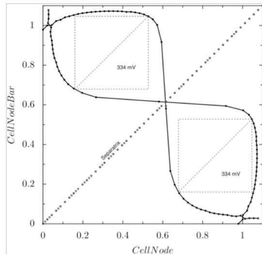
Figure 12. Nullclines and separatrix of a Portless 5T cell
