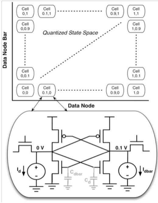
Figure 3. Quantizing the state space in the netlist
