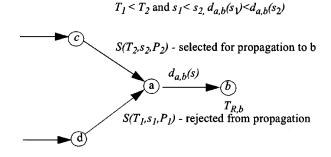
Fig. 9. Example of LPA underestimating node timing slack.
