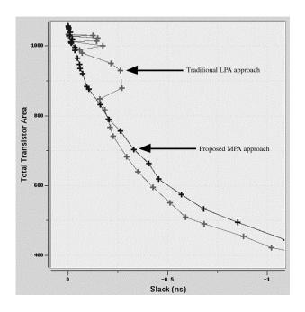
Fig. 13. Circuit optimization with LPA and proposed MPA methods.
