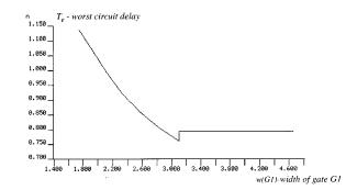
Fig. 2. Discontinuity in delay calculated by LPA method.
