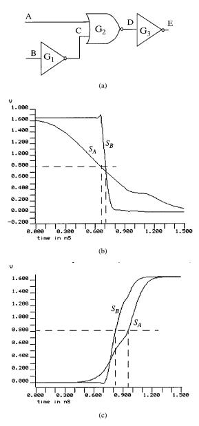
Fig. 1. Error in calculated circuit delay with LPA method. (a) Circuit with two signal propagation paths: A, D, E and B, D, E. (b) Waveforms of two signals at node D. Signal  $S_A$  originating from node A and signal  $S_B$  originating from node B. (c) Signals  $S_A$  and  $S_B$  after they propagate through gate  $G_3$ .
