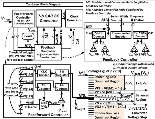
Figure 21.5.3: Top-level block diagram (top left). Feedback controller (top right). Feedforward controller (bottom left). Trigger voltages (bottom right):  $V_{target}$  can be generated by ultra-low power  $V_{ref}$  circuits [6-7].
