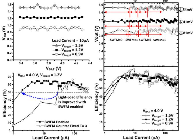
Figure 21.5.5: Measured  $V_{out}$  vs.  $V_{BAT}$  (top left). Measured  $V_{out}$ , and efficiency vs. load current (right). Measured efficiency vs. load current with SWFM enabled, and SWFM counter fixed to 3 (bottom left).
