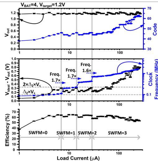
Figure 21.5.4: Measured results.  $V_{out}$  and code vs. load current (top).  $V_{ideal}-V_{out}$  and clock frequency vs. load current (middle). Efficiency vs. load current (bottom).
