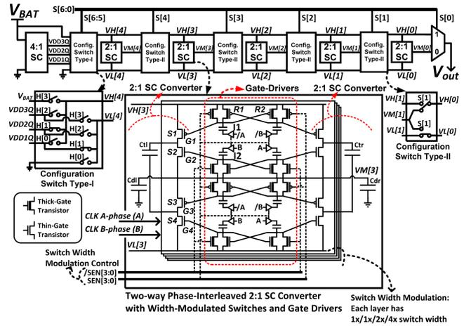
Figure 21.5.2: Schematic of the proposed 7-b SAR SC DC-DC converter (top). Detailed schematics (bottom).
