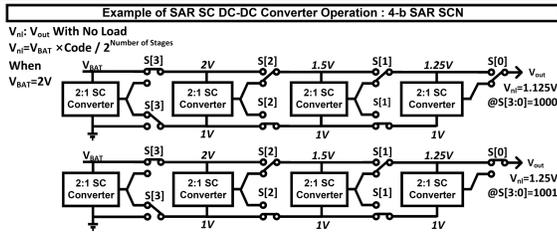
Figure 21.5.1: An example of 4-b SAR SC converter operation (top). Measured and ideal values of  $V_{out}$  vs. Code at  $V_{BAT}=4.0V$  under no-load condition for the proposed SAR SC converter (bottom).
