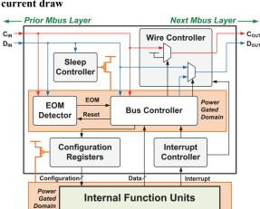
Figure 5. MBus design for low power IoT die-to-die communication
