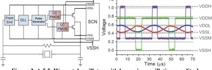
Figure 3. A 5.5nW crystal oscillator with low swing oscillation amplitude
