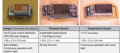
Figure 6. Millimeter sensor designs constructed using low power die connected through MBus
