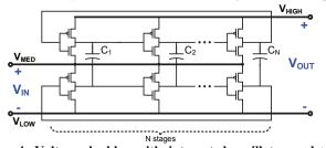
Figure 4. Voltage doubler with integrated oscillator and >70% efficiency from 1nA - 300µA
