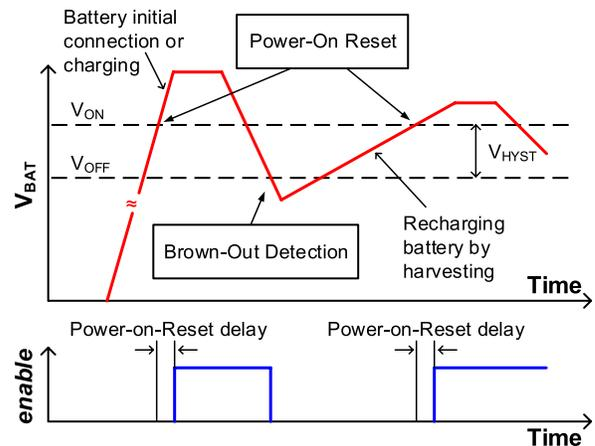
Fig. 2. Conceptual BVS operation according to  $V_{BAT}$ .
