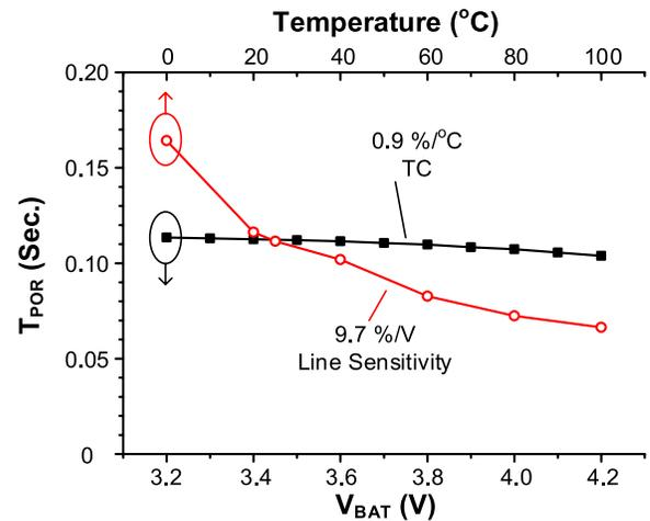
Fig. 27. Measured  $T_{POR}$  of AHBVS across temperatures and  $V_{BAT}$ .
