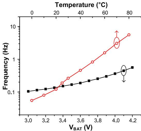
Fig. 23. Measured oscillator frequency across temperatures and  $V_{BAT}$ .
