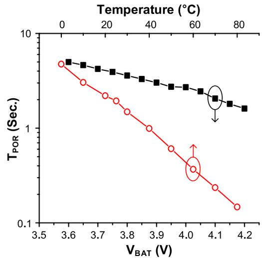
Fig. 22. Measured  $T_{POR}$  of LCHBVS across temperatures and  $V_{BAT}$ .
