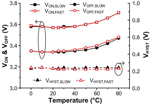
Fig. 19.  $V_{ON}$ ,  $V_{OFF}$ , and  $V_{HYST}$  across temperatures with different  $V_{BAT}$  transition speeds (0.25 mV/s and 0.8 V/ $\mu$ s).
