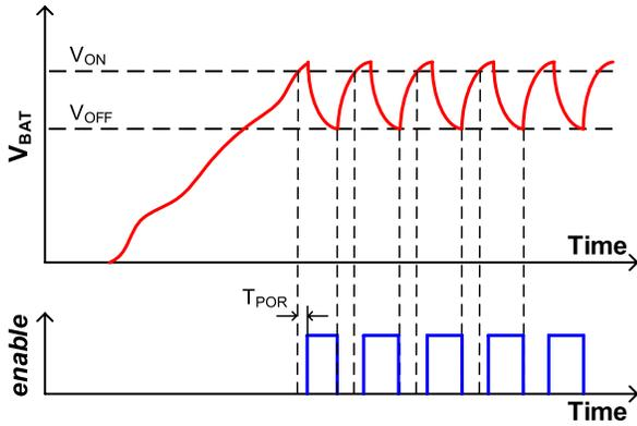
Fig. 3. System oscillation due to  $IR$  drop on  $V_{BAT}$  higher than  $V_{HYST}$ .
