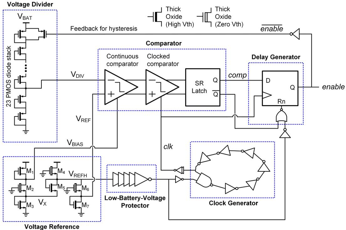
Fig. 6. Circuit diagram of LCHBVS.
