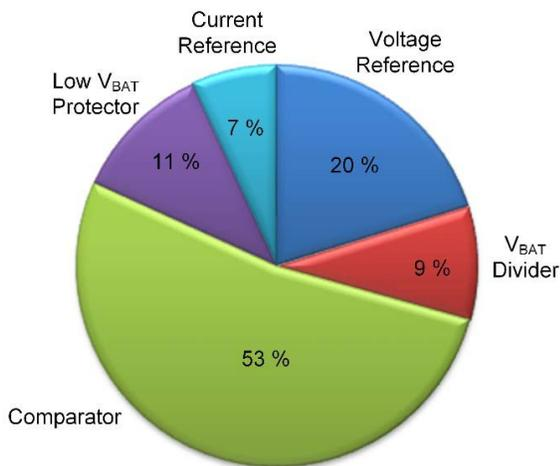
Fig. 25. Power breakdown of AHBVS.
