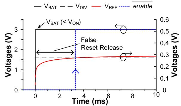
Fig. 8. False reset release using decoupling capacitor to ground in the conventional voltage reference.
