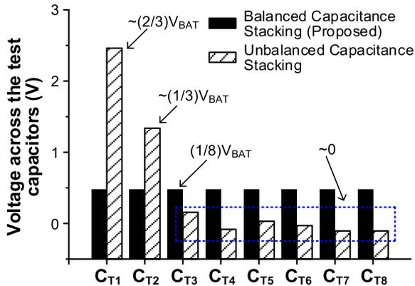
Fig. 15. Simulated voltages across test capacitors after discharging processes.
